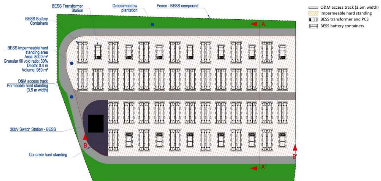
FIGURE 9.2 - INDICATIVE BESS LAYOUT
